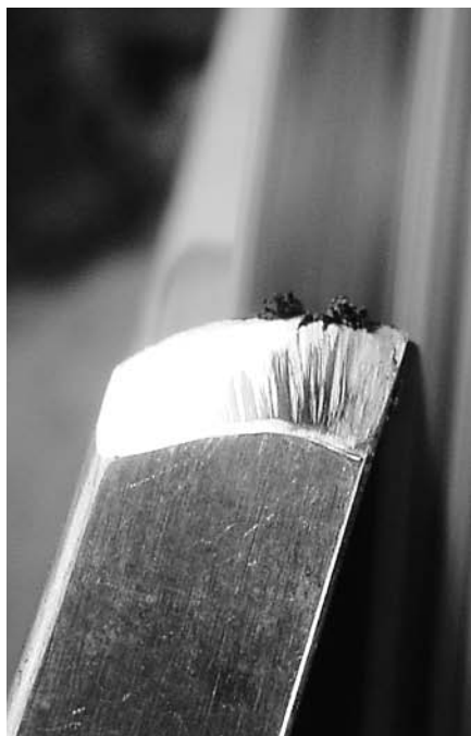
Watch for a "mud trail," shown above, when power-honing at an MDF wheel charged with honing compound.
