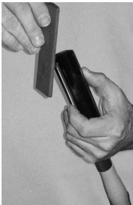
When honing, support the turning tool handle solidly against the body when honing. The grip above keeps the tool stationary.
